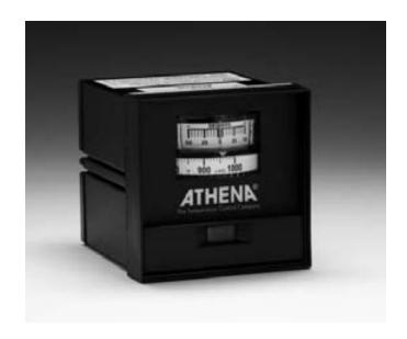
The Athena 2000 is a 1/4 DIN panel mounted, full featured, metal case enclosed controller that can be used for accurate proportional control of most processes. The Controller accepts thermocouple or RTD input and offers a choice of standard single outputs for energizing most common devices. A dual meter dial display provides visual indication of various controller functions.
