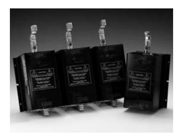
The Athena 19 and 39 controllers are available as zero voltage switched controllers (19Z and 39Z) and phase-angle fired controllers (19P and 39P) that can be used for control of resistive heater loads. The controller provides capacity up to 80 Amps, and extends heater life while eliminating thermal shock.
