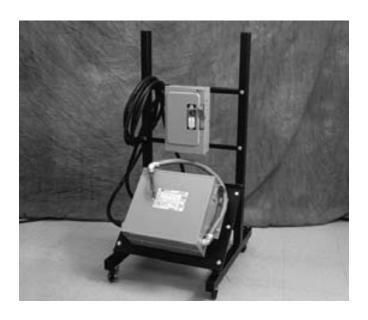
Transformer kits are fully wired and include enclosed transformer (480 Vac 3Ø in, 240 Vac 3Ø out) with adjustable voltage taps, power cable to main frame, disconnect switch, extra fuses, and floor stand with all hardware. Other transformers are available for your particular power requirements.
