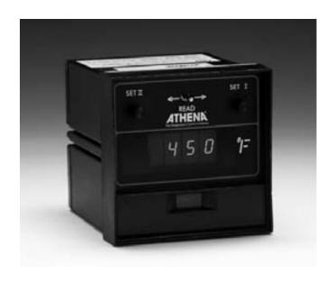
The Athena 4000 is a 1/4 DIN panel mounted, short metal case enclosed controller that can be used for accurate proportional temperature control of most processes. The controller accepts thermocouple or RTD input, and offers a choice of standard single outputs for energizing most common output devices. A single, digital filtered LED display provides visual indication of various controller functions.
