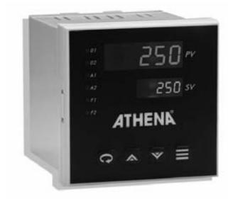
The Athena Legacy 25 is a 1/4 DIN panel mounted, auto-tuning controller that can be used for precise control of a single loop with two independent outputs. The controller accepts thermocouple, RTD, voltage, or current input. RS-232 or RS-485 communications are available, and two digital LED displays provide visual indication of various controller functions.
