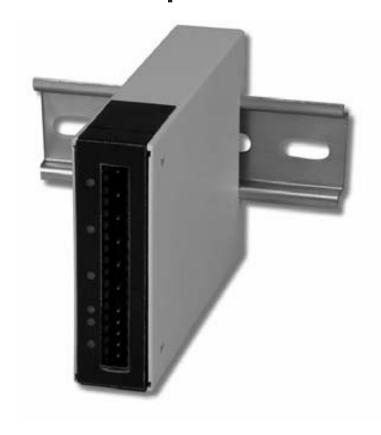
The Athena 1ZC is a DIN rail mounted, auto-tuning controller that can be used for precise control of a single control loop with two independent outputs configurable as direct-acting, reverse-acting or alarm. A bidirectional RS-485 serial communications interface is standard. Discrete LED displays become illuminated whenever associated outputs are active and provide system status. A wide range of sensor inputs are supported and many types of outputs are available.
