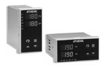
The Athena Legacy 18 and 19 Controllers are available as 1/8 DIN (18) vertical or 1/8 DIN (19) horizontal models. Both panel mounted, auto-tuning controllers can be used for precise control of a single loop with two independent outputs. The controllers accept thermocouple, RTD, voltage, or current input. RS-232 or RS-485 communications are available, and two digital LED displays provide visual indication of various controller functions.
