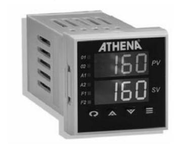
The Athena Legacy 16 is a 1/16 DIN panel mounted, auto-tuning controller that can be used for precise control of a single loop with two independent outputs. The controller accepts thermocouple, RTD, voltage, or current input. RS-232 or RS-485 communications are available, and two digital LED displays provide visual indication of various controller functions.
