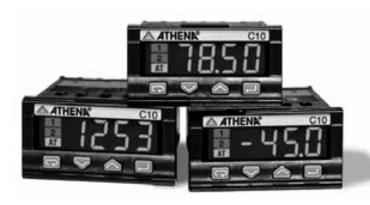
Athena's Platinum Series C10 is the smallest 1/32 DIN (48 x 24 mm) size panel-mounted line and combines all the functionality of a temperature controller-indicator-transmitter without losing the standard features found in more complex control devices such as auto-tune and IP65 front panel protection. Available options include serial communications, analog retransmission output, and transmitter power supply.
