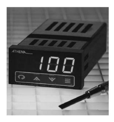
The Athena 32C is a 1/32 DIN panel mounted, autotuning controller that can be used for precise control of a single loop with two independent outputs field-configurable as direct acting, reverse acting or alarm. An LED display provides visual indication of various controller functions.
